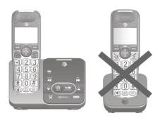
For registration, put the handset on the telephone base, not the handset charger.
