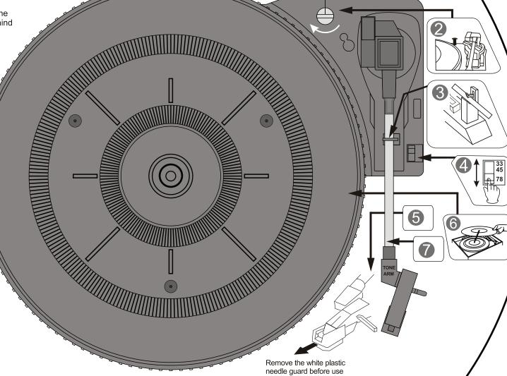
The tone arm will automatically stop at the end of the record. Then you must return the tone arm to the arm-rest manually.
