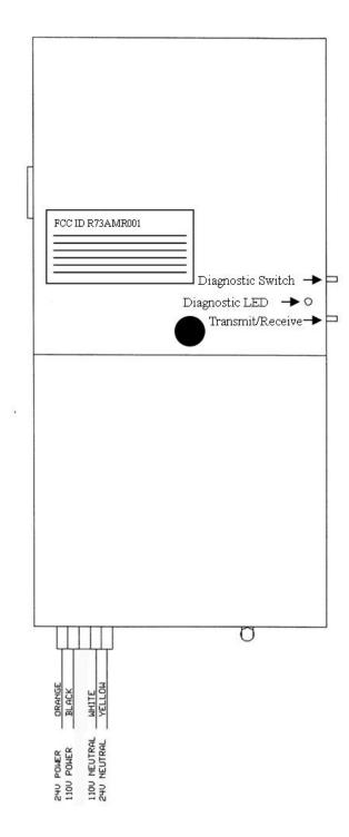
The V-AW12A and V-AW16A wireless clocks can be powered by 2 "D" cell batteries, 24 volts AC, 110 volts AC, or 220 volts AC.
